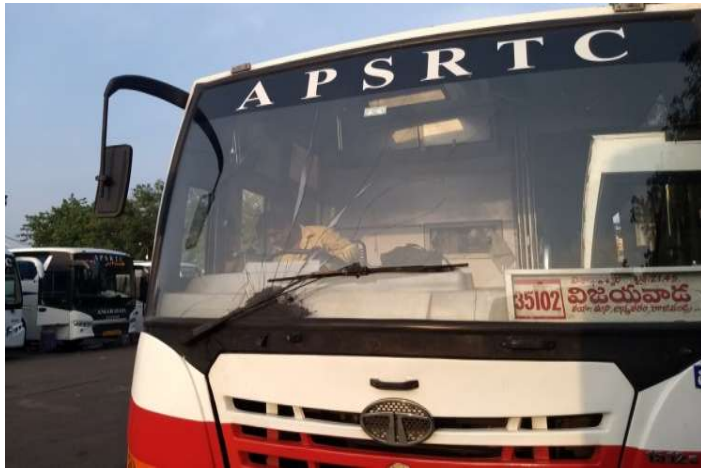
Fig.3 - Multiple cracks in front of driver
