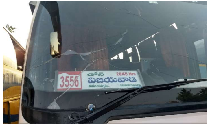
Fig.2- Multiple cracks and film separation
