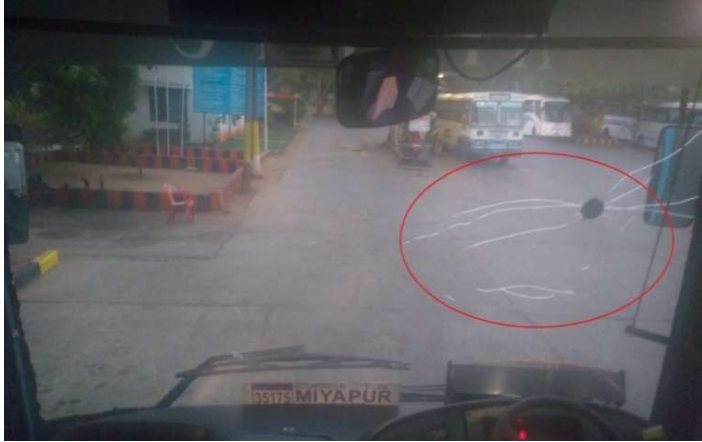
Fig. 1 – Cracks in front of Driver
